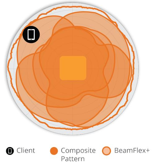
Figure 2. M510 2.4GHz Azimuth Antenna Patterns
