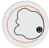
Figure 4. M510 2.4GHz Elevation Antenna Patterns
