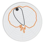
Figure 5. M510 5GHz Elevation Antenna Patterns
