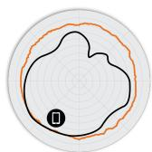
Figure 3. M510 5GHz AzimuthAntenna Patterns
