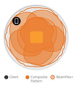
Figure 2. M510 2.4GHz Azimuth Antenna Patterns
