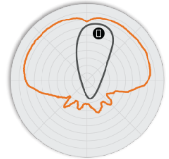
Figure 5. H320 5GHz Elevation Antenna Patterns
