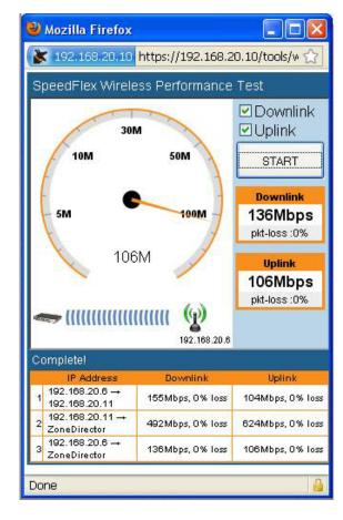
Figure 3: SpeedFlex™ is a unique wireless performance test tool integrated within the Ruckus family of centralized controllers that measures the Wi-Fi throughput of associated wireless LAN clients.
