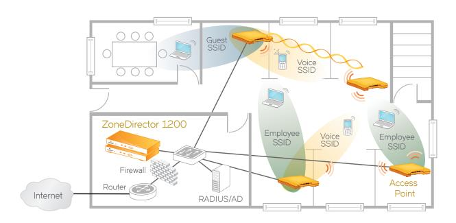
Figure 1: The ZoneDirector 1200 can be deployed anywhere within a Layer 2/3 network. All Ruckus APs automatically discover the ZoneDirector and are automatically provisioned.
